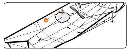
The bow bulkhead stays in the kayak. Hook it onto the gray ring strap as shown. This keeps the bulkhead and footrest safely out of the way when folding up the kayak
