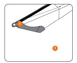
1 Moving from bow to stern, unclip the fairings and remove the foam plug.
