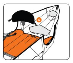
Remove seatback, seat pad and both stern bulkheads.
