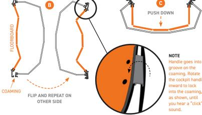
aroove on the coaming. Rotate the cockpit handle inward to lock into the coaming, as shown, until vou hear a "click"
