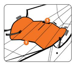
Remove the floorboard by lifting up from the center sides on the rubber trim indicated in the illlustration above. Do **not** use the bungee to remove the floorboard.
