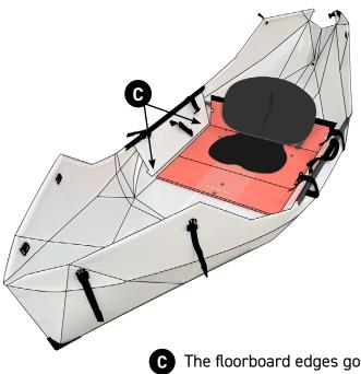
The floorboard edges go in the gaps between the sideboards and the bottom of the kayak.
